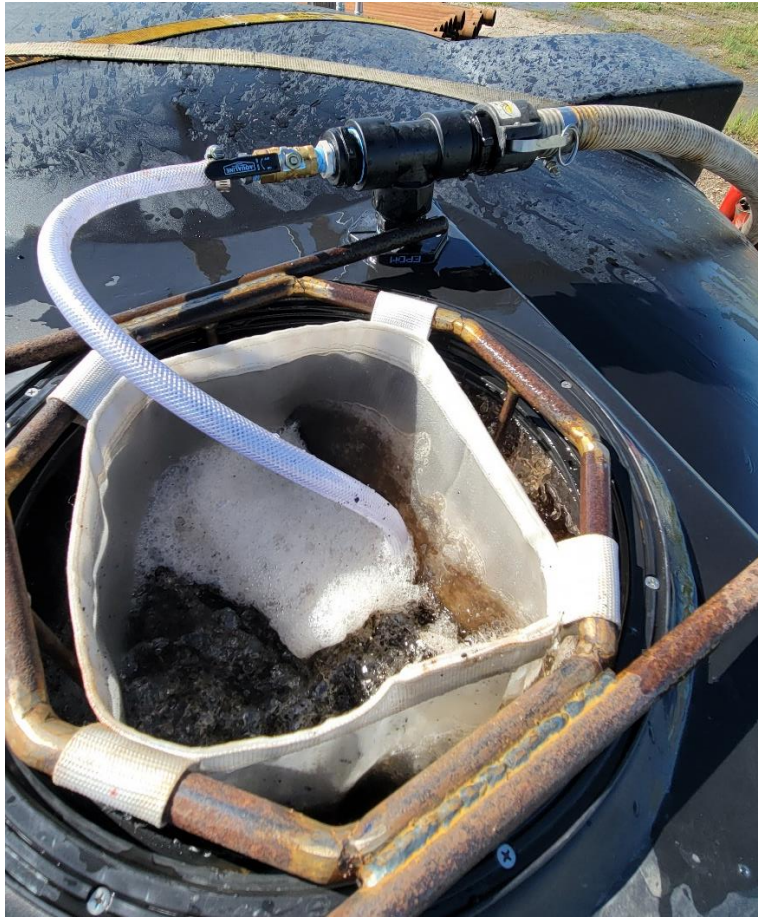
The basket is manufactured to fit a standard manhole, with the bag made to fit.
