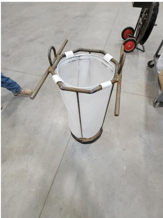
The basket is manufactured to fit a standard manhole, with the bag made to fit.
